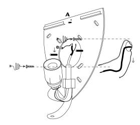
4. Place the metal plate **B** over element **A** so that the threaded studs extends through the 2 holes. Secure against the mounting surface using the 2 mounting caps **C** provided.
