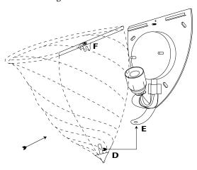
6. To secure the fixture against the mounting surface hang the element **F** to the mounting bracket as shown. Turn the hook **G** and fix it using the screw **H**.
