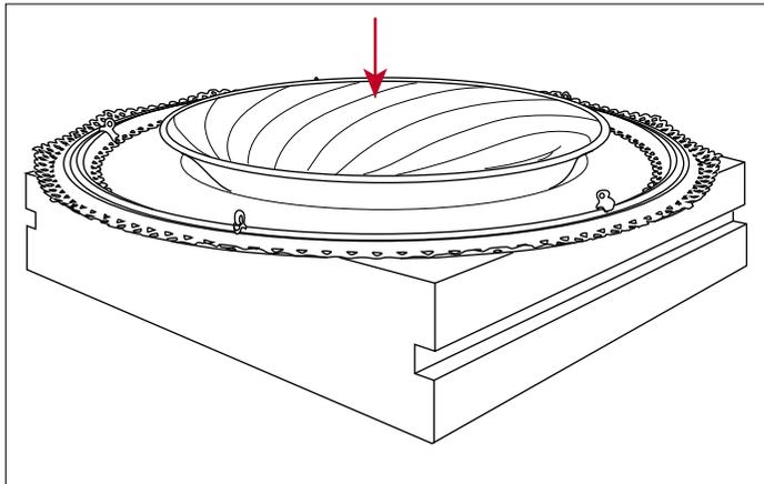
11/12. Fix the 5 pins **E** by means of the screws **F**
