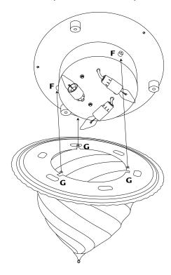
7. Suspend the drop. Restore the electricity and test.
