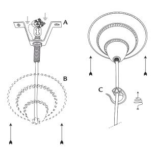
5. Screw the hook **C** onto the nipple and tighten securely.
