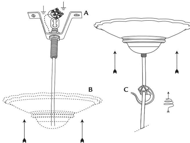
5. Screw the hook **C** onto the nipple and tighten securely.
