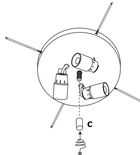
6. Install bulbs. Do not exceed the maximum wattage for this fixture. Refer to the wattage warning label attached to the fixture for maximum allowable wattage.
